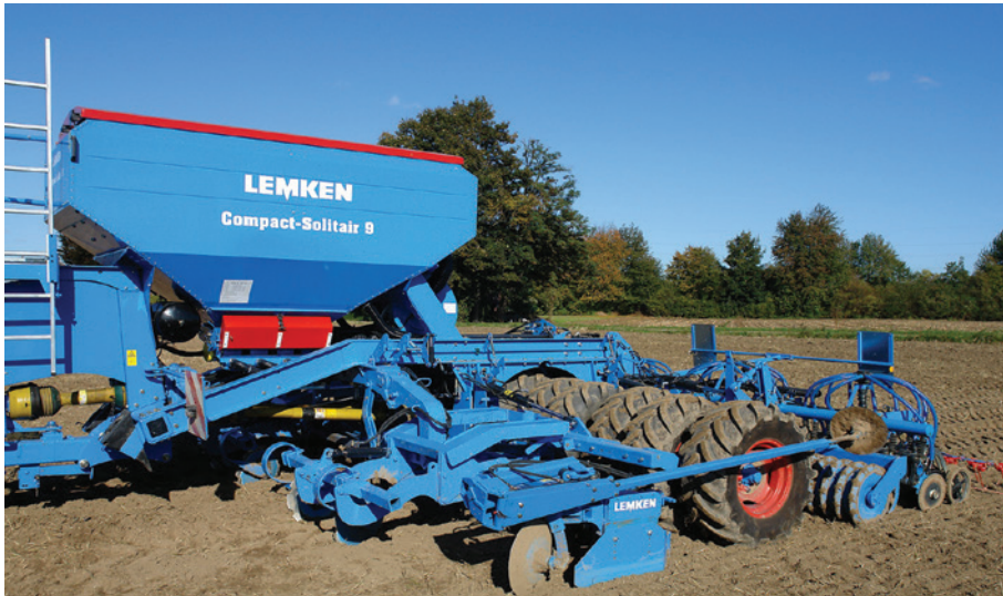
The narrower AC 65 N tyre has been designed for special agricultural machinery like seeders and is supplied in the 420/65R20 size.
